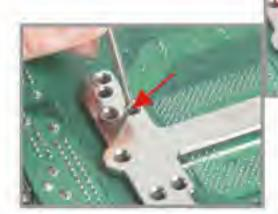
Turn to front side of the motherboard and place the washers on to the four screws.
